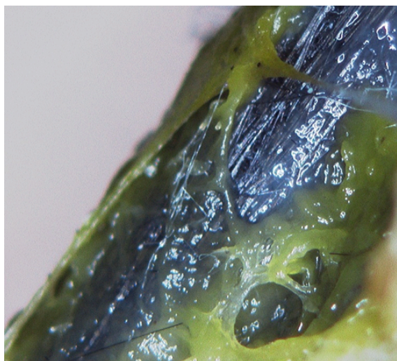
Figure 6. P. polycephalum colonising the cathode electrode (50x magnification, Hirox Europe Ltd, Limonest, France). The carbon veil electrode appears glossy and wet due to the presence of the protoplasm generated by P. polycephalum .
